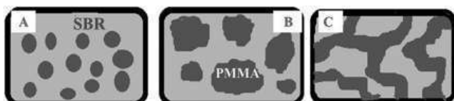
Figure 2.3: Schematic representation showing the effect of concentration of second component in morphology of resultant S-IPN, (A) S-IPN with low PMMA content, (B) moderate PMMA content and (C) high PMMA content
