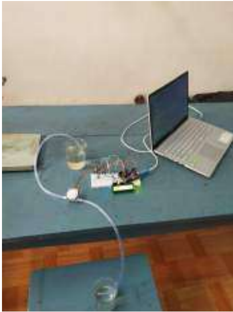
Figure: Automated setup for measuring viscosity
